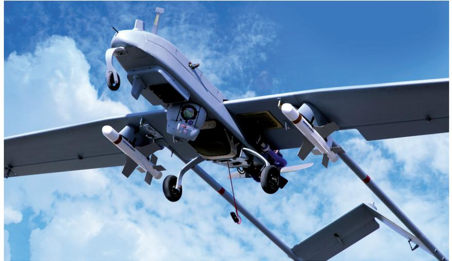
Fury is a small, lightweight glide weapon designed for and integrated onto tactical unmanned aircraft system (TUAS) platforms, including the Textron Systems Unmanned Systems Shadow® and Shadow M2.
