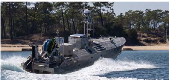
The CUSV® performs at a NATO demonstration integrated with the Towed Reelable Active/ Passive Sonar (TRAPS) anti-submarine payload.
