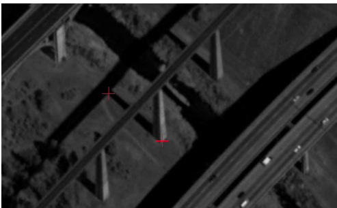
Height (185 feet) determined using Shadow Height tool.
