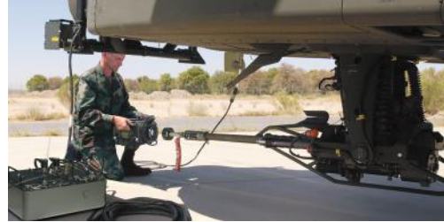
ABE easily aligns the Apache® area weapon system using a small adapter. The need for an unobstructed line-of-sight between the aircraft reference and the stations is eliminated.
