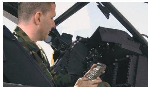
The portable HHDU allows an operator to view boresight results at any location. ABE is designed to align systems on any land, sea or air vehicle.
