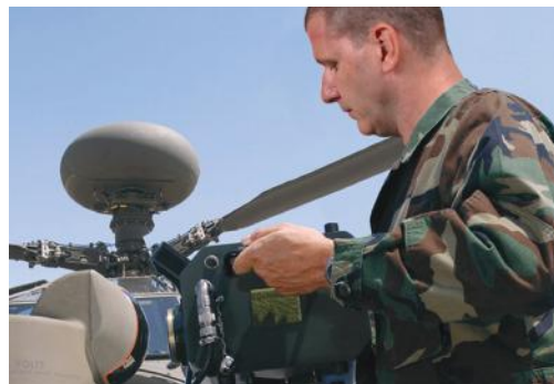
ABE projects accurately aligned infrared or visible images into optical sensors, eliminating the need for station-unique adapters for most optical systems.
