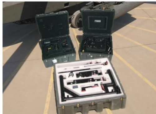
The ABE field boresight system for Apache helicopters is contained in three compact, rugged, easily transportable transit cases.
