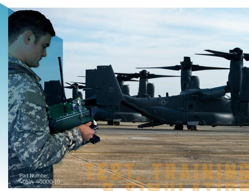
The Integrated Tester for Aircraft Survivability Systems (ITASS) verifies radar warning receivers, missile warning systems, laser warning systems and other radio frequency (RF) systems onboard aircraft, providing operators the tools they need to confidently validate the operational status of the systems.
