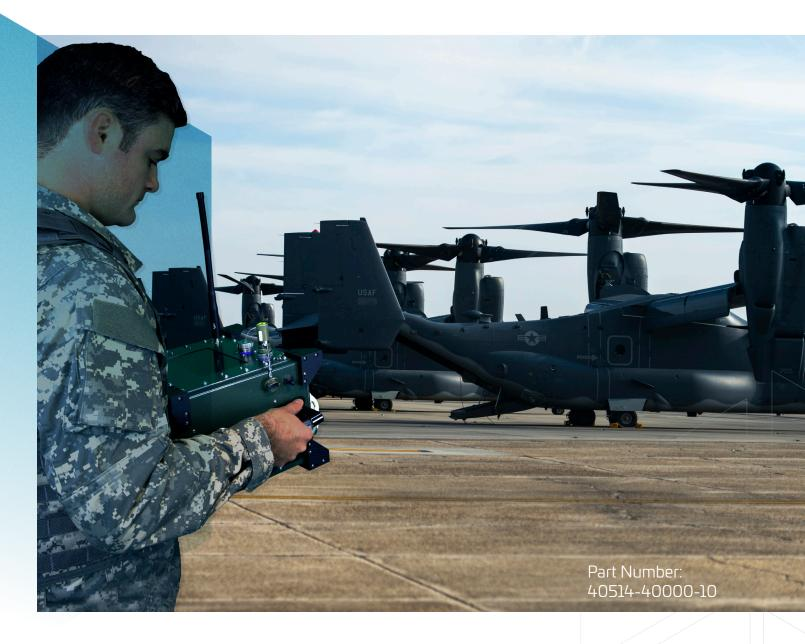
The Integrated Tester for Aircraft Survivability Systems (ITASS) verifies radar warning receivers, missile warning systems, laser warning systems and other radio frequency (RF) systems onboard aircraft, providing operators the tools they need to confidently validate the operational status of the systems.
