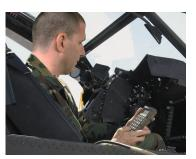
The portable HHDU allows an operator to view boresight results at any location. ABE is designed to align systems on any land, sea or air vehicle.
