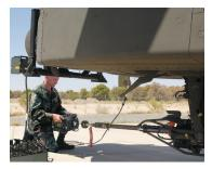
ABE easily aligns the Apache® area weapon system using a small adapter. The need for an unobstructed line-ofsight between the aircraft reference and the stations is eliminated.
