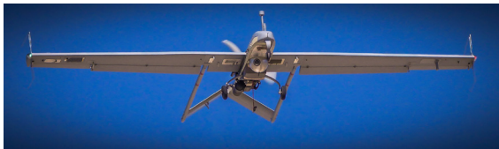
The Shadow Block III upgrade provides an HD payload and increased engine reliability.
