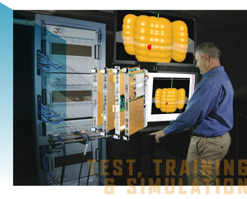
The -150 SSI is the next generation SSI (Synthetic Stimulus Instrument). The -150 SSI is a phase-coherent, wide-band Direct-Digital Synthesizer (DDS), which provides 500MHz of instantaneous bandwidth, enabling threat generation of today's most complex emitters. The two modes of operation enable the capability to generate 2 MPPS in radar mode or 20 simultaneous communication emitters per -150 SSI, creating a dense, complex, realistic environment for test and evaluation.
