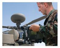
ABE projects accurately aligned infrared or visible images into optical sensors, eliminating the need for station-unique adapters for most optical systems.
