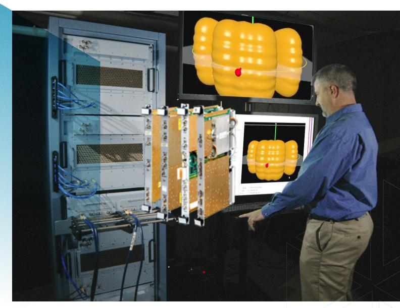
The -150 SSI is the next generation SSI (Synthetic Stimulus Instrument). The -150 SSI is a phasecoherent, wide-band Direct-Digital Synthesizer (DDS), which provides 500MHz of instantaneous bandwidth, enabling threat generation of today's most complex emitters. The two modes of operation enable the capability to generate 2 MPPS in radar mode or 20 simultaneous communication emitters per -150 SSI, creating a dense, complex, realistic environment for test and evaluation.
