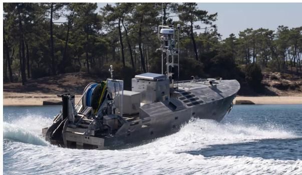
The CUSV® system performs at a NATO demonstration integrated with the Towed Reelable Active/ Passive Sonar (TRAPS) anti-submarine payload.
