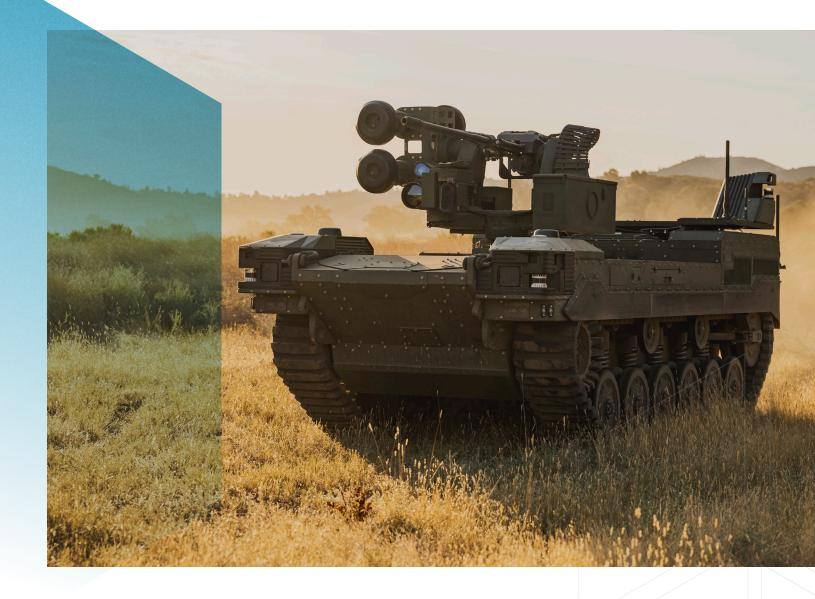
The RIPSAW® M3 Robotic Vehicle is the newest generation platform within the RIPSAW family of vehicles. The RIPSAW M3 incorporates the familiar large, open deck area from the RIPSAW M5 robotic vehicle and 10kW of offload power provides the flexibility to support multiple lethality, RSTA, combat engineering and logistics payloads. With a powerful hybrid electric drivetrain and novel suspension, the RIPSAW M3 provides unmatched mobility with over 180 miles of range.
